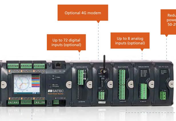
Redundant aux. AC/DC power supply (optional) 50-290V AC (50/60 Hz), 40-290V DC
