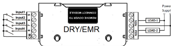
Figure 2-13 Dry Contact Inputs Connection
